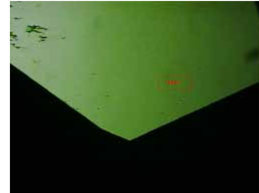
„Third cutting edge“ – break in crystal structure
