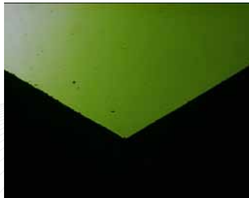
Chipping cutting edges caused by wrong diamond maintenance e.g. cleaning by brush, compressed air or kneading rubber
