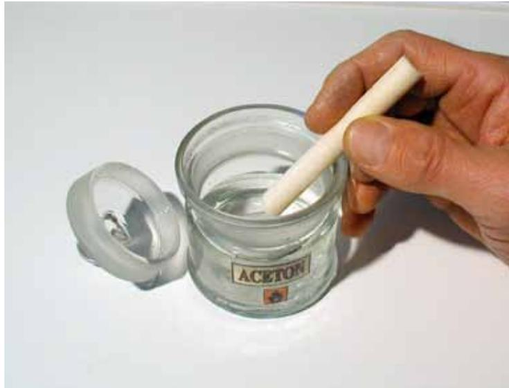
Freshly cut front part of the elder pitch has to be briefly dipped into acetone and is then ready to be used for cleaning the diamond.
