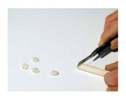
Make sure that the contact surface of the elder pitch is cleaned from contaminations at all time.
